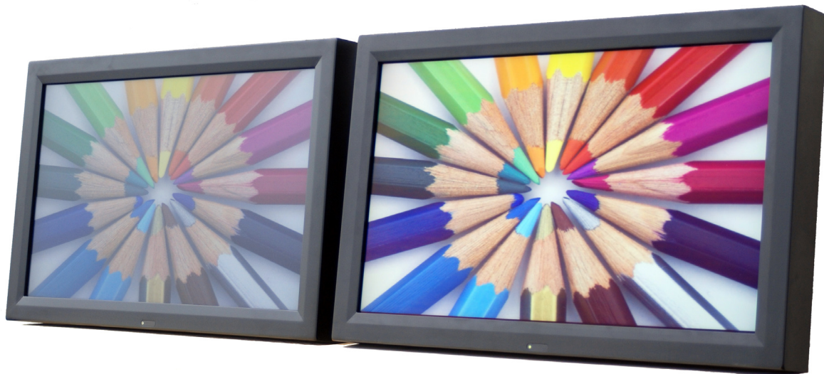
Regular LCD screen versus Transreflective LCD screen exposed to direct sunlight.
